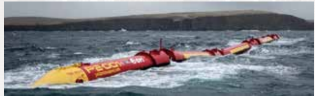
Fig. 1. Pelamis wave energy converter. Source: EMEC website [4]
