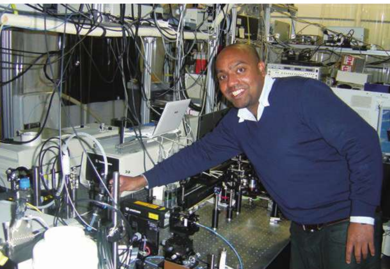
Aligning an optical measurement system which is used to evaluate device characteristics
