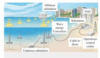
Figure 1 A typical WEC arrangement
